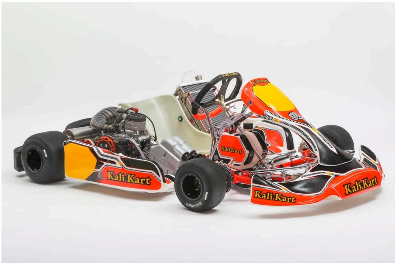
**KZ CHASSIS.** The centre of gravity of the competitive KK 04 model has been modified in function of the tyres used in the main KZ categories, which improved cornering, braking and traction. Performance has also been optimized by a slight change in the rear track. The KK 04 model feature magnesium R-line hubs and spindles, magnesium wheels and new VEN 11 KZ braking systems, developed by the CRG's research and development centre.
